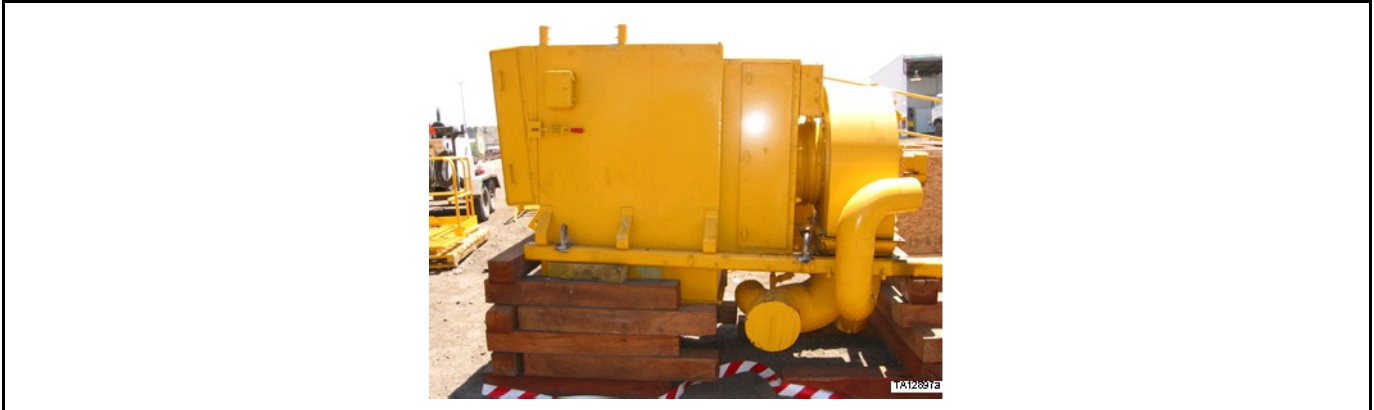
Figure 15: KLENZ™ and blower assembly supported by cribbing - 1 of 3
