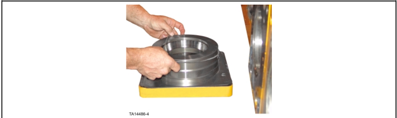
Figure 21: Installation of O-ring to rear output bearing housing
