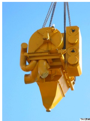
Figure 14: Hoisting of KLENZ™ and blower assembly
