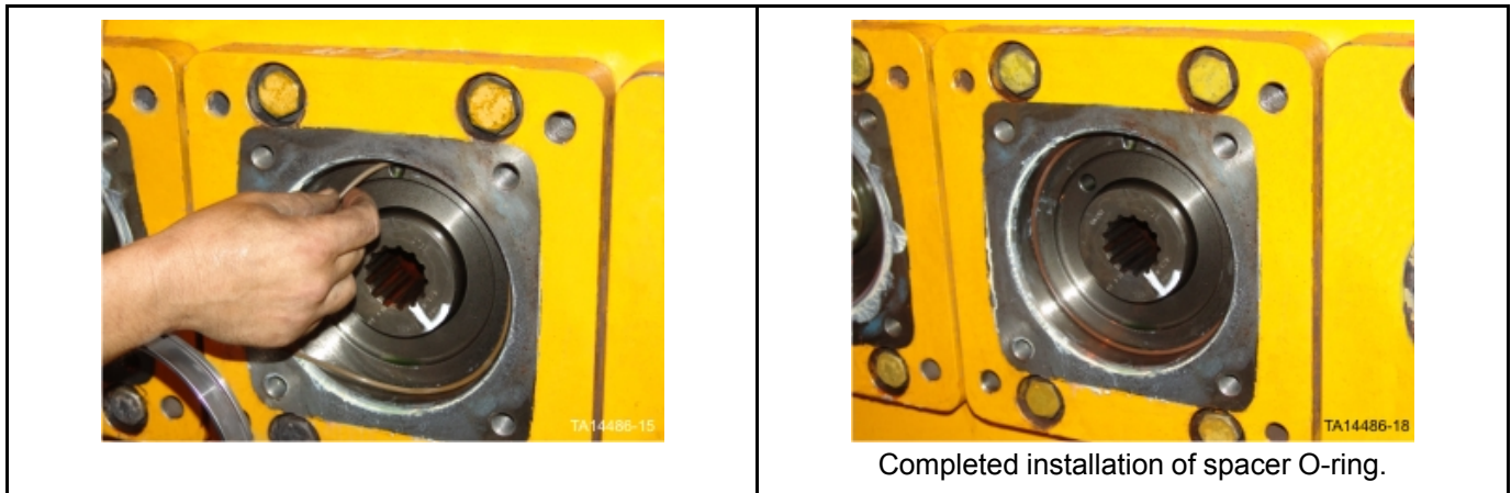
Figure 34: Installation of spacer O-ring into output bearing housing
