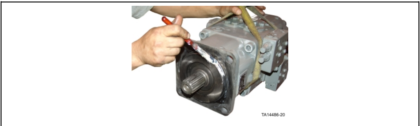
Figure 38: Application of assembly grease to pump O-ring and pump.
