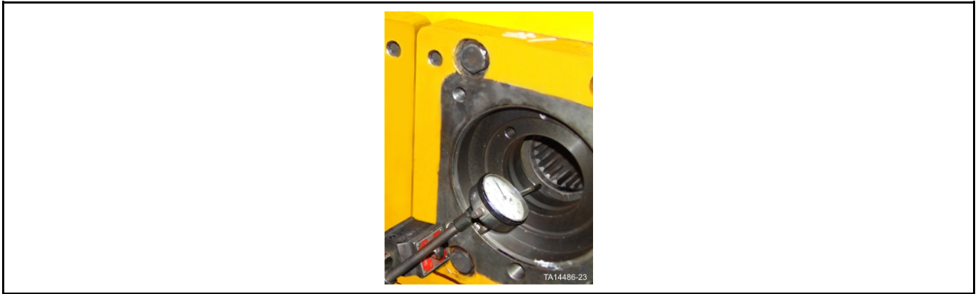
Figure 26: Magnetic base dial indicator in position to read bearing end play
