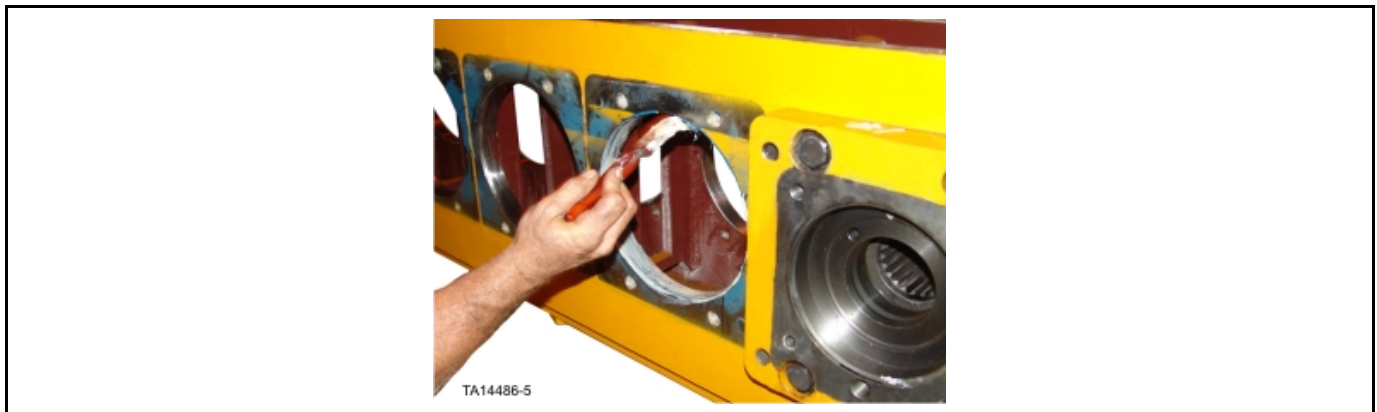
Figure 22: Application of assembly grease to gearbox
