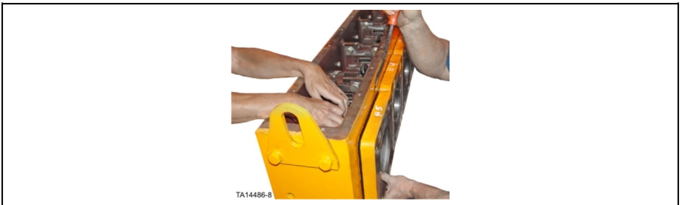
Figure 29: Removal of front output bearing housing for shim adjustment
