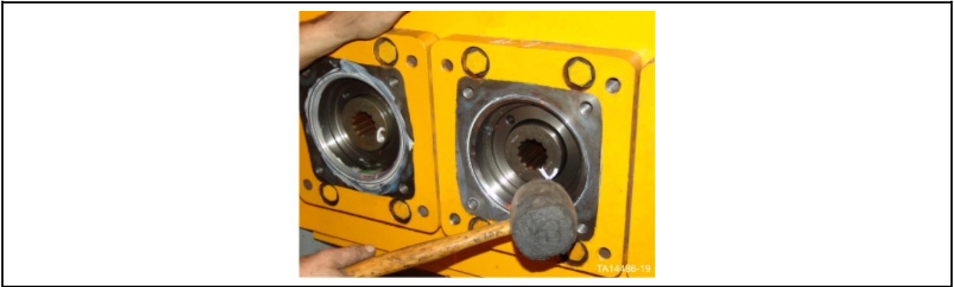
Figure 37: Installation of sleeve into output bearing housing
