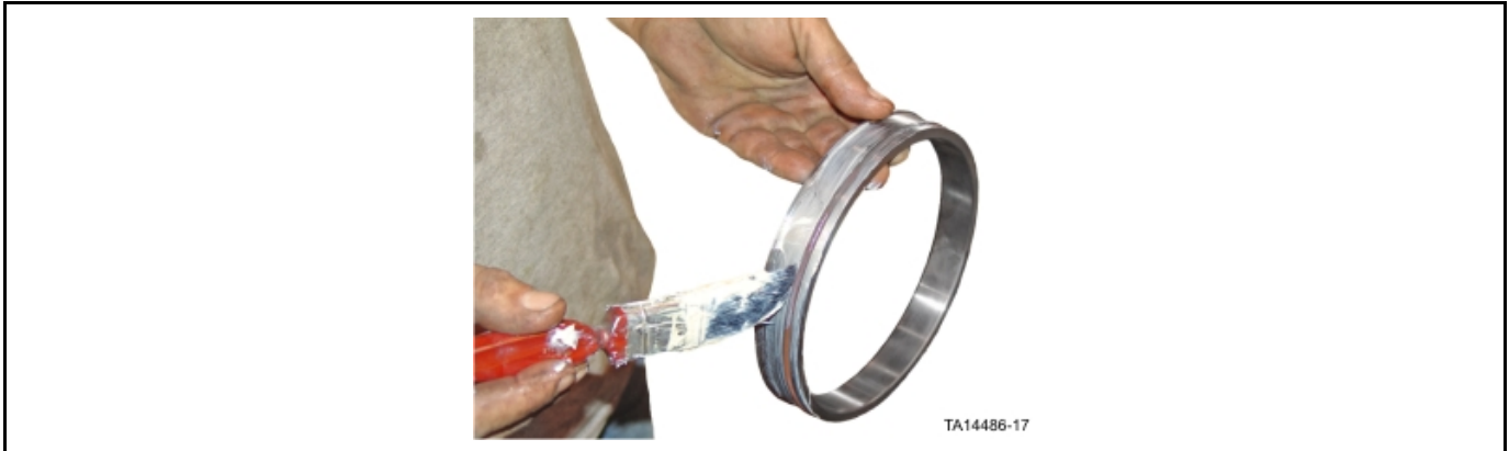
Figure 35: Application of assembly grease to sleeve O-ring and sleeve.
