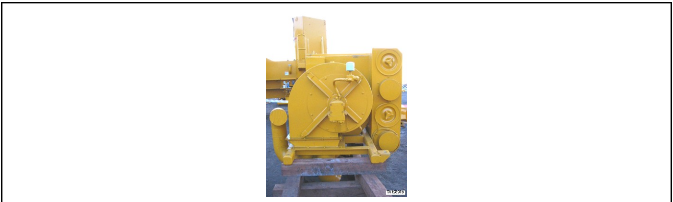
Figure 16: KLENZ™ and blower assembly supported by cribbing - 2 of 3
