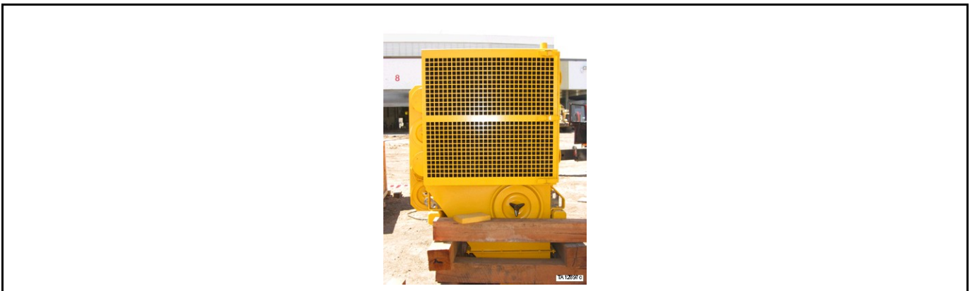
Figure 17: KLENZ™ and blower assembly supported by cribbing - 3 of 3
