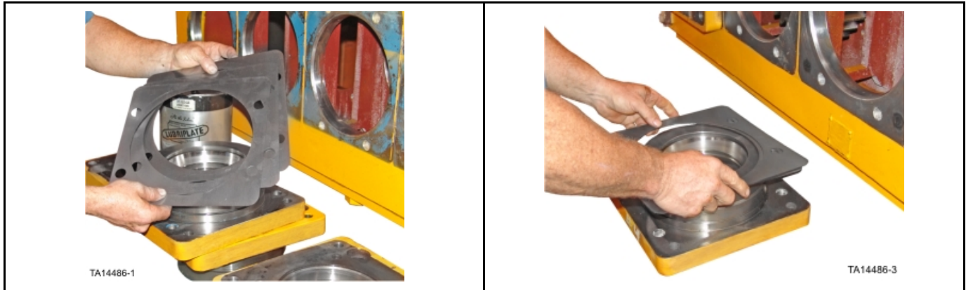
Figure 19: Three .020 shims to be installed to rear output bearing housing Figure 24: Installation of shims (.060) to rear output bearing housings
