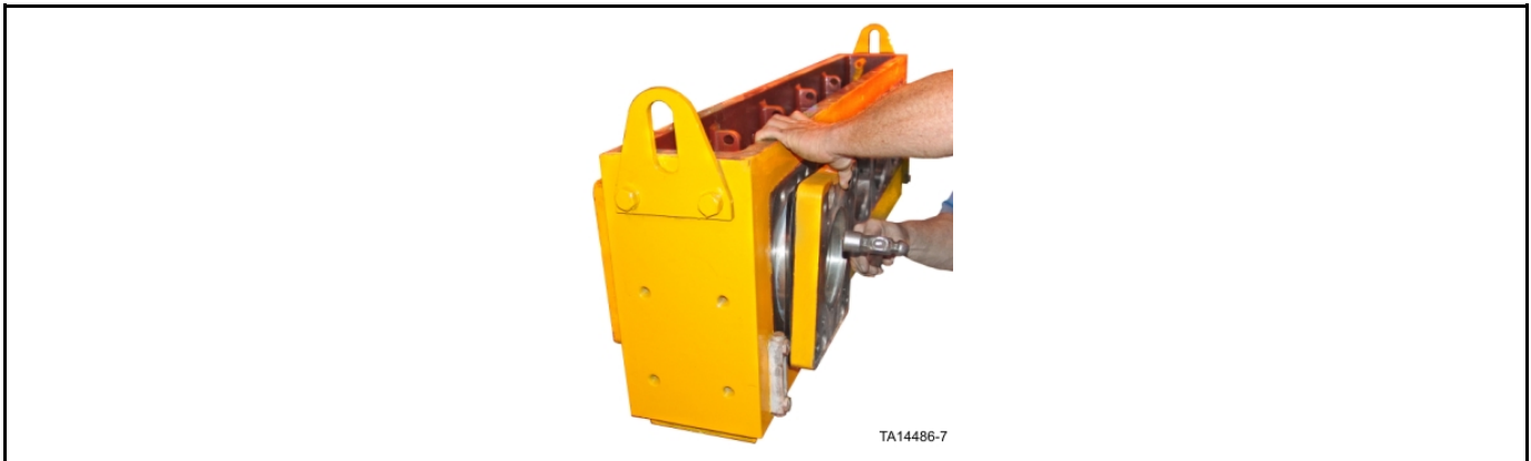
Figure 24: Installation of front output bearing housing with .040 shims in place
